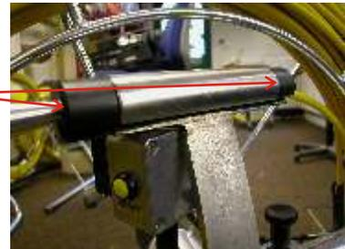
For transportation purposes the camera spring and rod maybe withdrawn from the meterage device and inserted into the reel.
