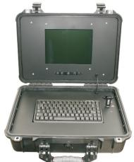
The CS550 may be powered using Mains 100-230Va.c supply. Sourced from mains, Inverter or generator. !! Warning !! :- Some poor or unregulated generators may permanently damage this equipment. Check regulation, leads and earthing before use.
